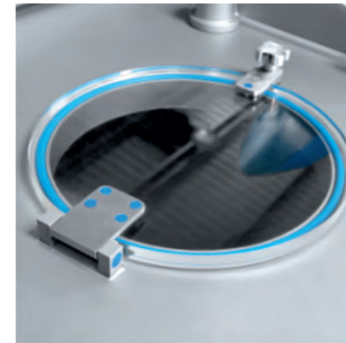
THE CHECK OPENING HOLE IN THE BOWL COVER ABERTURA DE CONTROL EN LA TAPA
